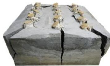
Cracking up the concrete (after few hours)
