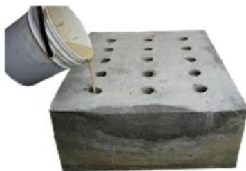
Filled up with Tii-Conbreak slurry
